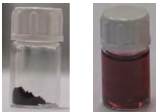
Fig. II.11. FLG powder (left) and its dispersion in cell culture medium (right).
