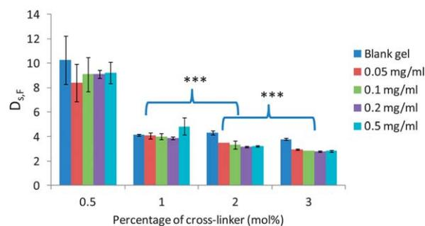
**Fig. 2** Swelling properties of the hybrid gels. The final swelling of the gels was expressed as  $D_{s,F}$ , measured when the gels reached a constant weight and plotted versus the cross-linker concentration for all hybrids.
