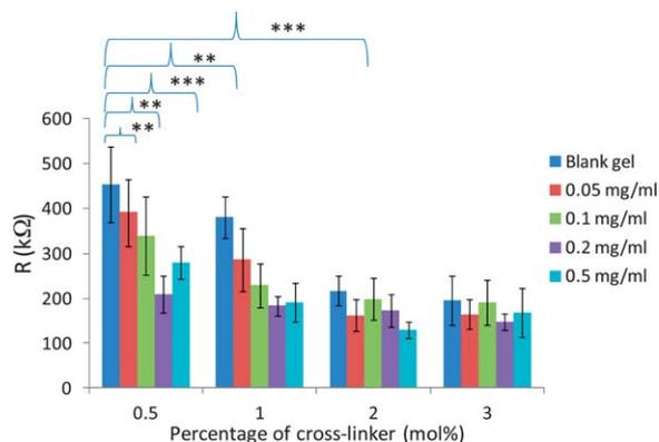
**Fig. 3** Characterisation of the electrical conductivity of the hybrid gels: bulk resistivity  $R$  of all hydrogel hybrids of a volume of 1 cm<sup>3</sup> at different cross-linker concentrations (from 0.5 mol% to 3 mol%): the bulk resistivity was determined as the product between the thickness of the sample and the sheet resistance  $R_s$ .
