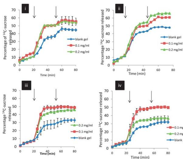
**Fig. 6** Pulsatile drug release from hydrogel hybrids upon the on/off application of an electrical voltage. The pulsatile release of <sup>14</sup>C-sucrose was determined for the blank gel and the selected hydrogel hybrids (0.1 mg ml<sup>-1</sup> and 0.2 mg ml<sup>-1</sup> of MWNTs) at: (i) 0.5 mol%, (ii) 1 mol%, (iii) 2 mol% and (iv) 3 mol% of cross-linker. The black arrows indicate when the electric field is switched on. The electric field is then switched off after 15 min.
