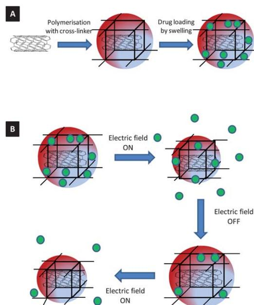
**Scheme 1** pMWNT-PMAA hydrogel hybrids for pulsatile drug release. (A) Preparation of the pMWNT-PMAA hydrogel hybrids: methacrylic acid (MAA), *N,N'*-methylene bisacrylamide (BIS) and potassium persulfate were used as a backbone monomer, a cross-linker and an initiator, respectively. (B) Pulsatile drug release upon electrical stimulation.
