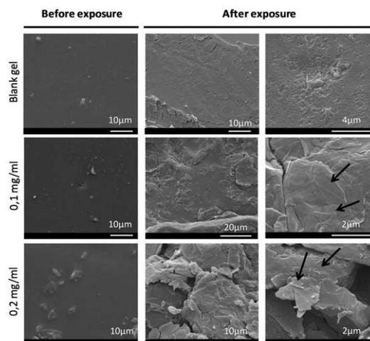
**Fig. 7** Effect of electrical exposure on the gel microstructure: SEM images of the hybrid gels before and after exposure to the electrical voltage; blank gel, 0.1 mg ml<sup>-1</sup> of MWNTs, 0.2 mg ml<sup>-1</sup> MWNTs at 1 mol% of cross-linker. The exposure to the electrical voltage led to significant structural damage of the hybrid gels compared to the blank gel.
