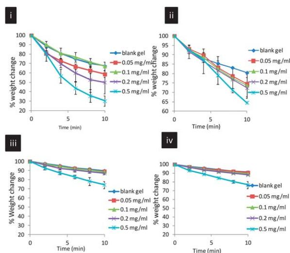
**Fig. 5** Gel response upon exposure to an applied electrical voltage (10 V); de-swelling of hydrogel hybrids upon the application of an electrical voltage. Water release from the gel matrix corresponding to the percentage weight change of the gels was monitored over time for all hydrogels prepared at different cross-linker concentrations: (i) 0.5 mol%, (ii) 1 mol%, (iii) 2 mol% and (iv) 3 mol%.
