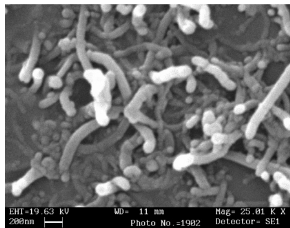
Figure 3. SEM image of the sensor chip functionalized with MWNT-NH 3 + ( 2 ).
