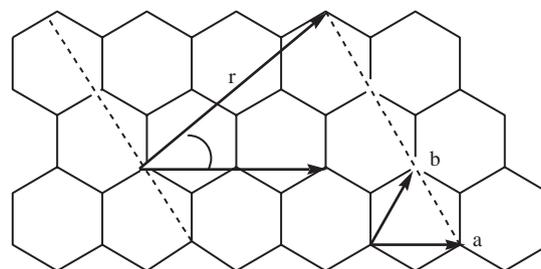
**Fig. 2.** Scheme to create the nanotubes cylinders from planar graphene sheets:  $\mathbf{a}$  and  $\mathbf{b}$  are primitive vectors of the hexagonal lattice,  $\mathbf{r}$  is a roll-up vector.
