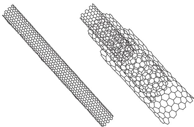
**Fig. 1.** Molecular structures of CNT fragments: (left) SWNT and (right) MWNT. The distance between the MWNT graphene layers is 0.34 nm.
